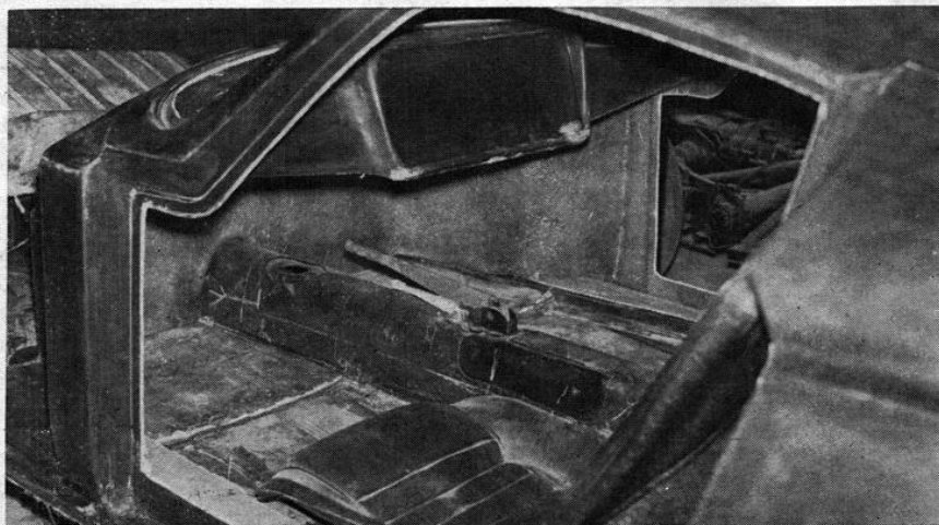
Cutting out windows and doors, above left, is quick procedure. Glass is easily fitted, right, with use of adhesives. Interior doesn't look like much now, below, but will be padded, carpeted.
